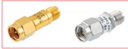
▲ Fig. 6 PE7467-10 (gold-plated brass) and PE7602-10 (stainless-steel) fixed attenuator pads.
